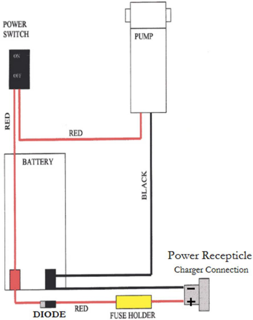
DIODE MUST BE INSTALLED WITH GRAY STRIPE TOWARDS BATTERY
